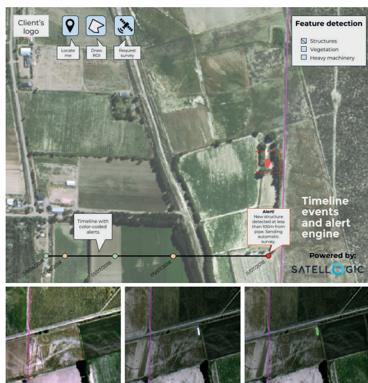
Before, after and semantic change detection results (new man-made structure)
