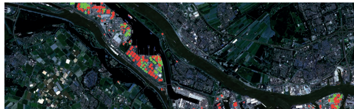
Detection of storage tanks (green) and oil storage tanks (red)
